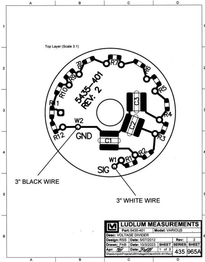
2 inch Voltage Divider Board - Schematic
