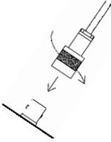
Connect one end of the cable provided to the detector by firmly pushing the connector together while twisting clockwise a quarter of a turn until latched. Repeat the process in the same manner with the other end of the cable and the instrument.
