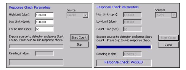
When the test is complete, the final activity reading and results of the test are displayed with a Pass/Fail possibility. In the event of a **Response Check: FAILED**, it is up to the user to determine whether the instrument is still serviceable. As with any statistical test, given a
