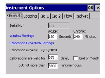
**Serial No—**This is a *non-editable* field that identifies the factory-defined serial number of the Model 334A. *Default: Factory set*.
