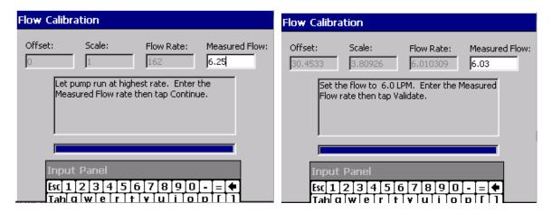
The flow calibration is now completed and this example shows 0.4% error, which is acceptable. Tap **Close**, and when prompted, "Do you want to save the changes?" click **YES**. Remove the flow calibration aid from the detector head, which may be difficult because of the suction created. It is recommended that the pump is turned off temporarily for better leverage. Lastly, replace the filter and close up the detector head.
