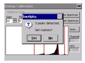
You can always manually set the markers by lining up each of the red lines with their respective peak location. Tap on a line and drag it across the screen until they line up with
