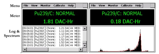
The **Menu** bar across the top of the screen provides access to the various settings and other information. They will appear differently depending on whether the password security feature is enabled. These menu items and their sub-menus will be covered in detail in other sections of the manual.
