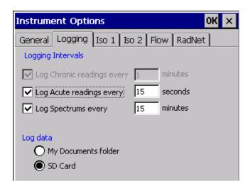
**Log Chronic readings every**—This setting controls the frequency in minutes that Chronic readings are written to a log file (e.g., Pu239\_ChronicYYYYMMDD.txt). Each file name has the format NameYYYYMMDD.txt, where YYYY represents the year, MM represents the month, and DD represents the creation day. If this setting is checked, the frequency field will be enabled. This setting defines the frequency in minutes that readings are time-stamped and logged. *Default is 1 minute*.
