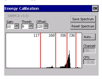
The horizontal axis represents the possible energies, assigned to channels 0 to 255. The vertical scale accumulates counts in each channel and adjusts automatically to display the highest peak.
