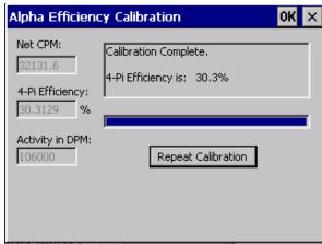
After the calibration has completed, it will report the efficiency. Typical 4pi efficiency should be around 30%. Typical efficiencies are 25-31% for Am-241. If the efficiency falls outside these parameters, either **Repeat Calibration** or call a Ludlum Technician for assistance.
