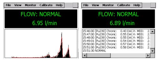
In the event that a dose or concentration reading exceeds alarm limits, the Model 334A will alarm visually and audibly, automatically display the channel of the chronic or acute reading that caused the alarm, and the status will be changed to **High Alarm**.
