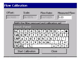
The first step in the flow calibration is to reduce the flow rate by adjusting the flow restriction device to a low flow rate, at about **2 LPM below** the unrestricted rate. Enter the actual value from the flowmeter in the dialogue under *Measured Flow*, and then hit **Start Calibration**. Each step in the process will take about 30 seconds as indicated by the progress bar. Repeat this process at about **1 LPM** below the unrestricted rate.
