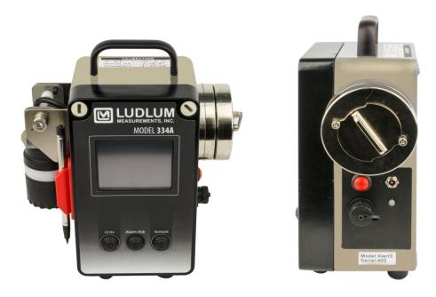
On the front, the Model 334A contains a 5.5-inch touch-screen display. The display is most easily operated using a stylus. There are three buttons located below the touch-screen display, which allow the user to toggle displayed units and channel, as well as an alarm acknowledge to silence and clear an alarm.
