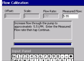
In the third step, adjust the flow restriction device until it is completely open, providing maximum flow. Again, input the LPM indicated on the flowmeter into the *Measured Flow* box on the screen. Continue with the same process as before.
