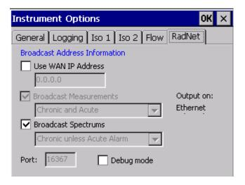
**Use WAN IP Address**—When checked, a specific WAN IP address can be entered. When unchecked, the unit broadcasts to the entire C-class subnet. *Default is unchecked*
