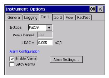
**Isotope**—This pull-down list provides for the selection of other isotopes of interest from the user-editable **Isotopes Database**. This selection affects only the isotope of interest and not the measurement of radon daughters, which are always monitored. *Default is Pu-239*.
