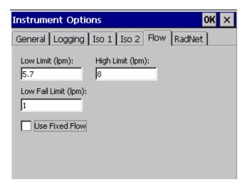
**Low Limit**—This setting defines the limit in liters per minute below which the Model 334A will indicate a LO FLOW status. A low flow status can indicate a loaded or wet filter. *Default is 6.0 LPM*
