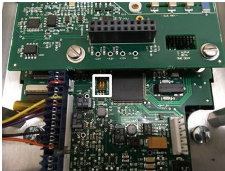
Figure 4.1: Backlight/Setup Protect Dipswitch
