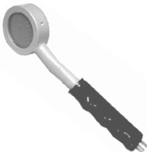
The response kit GM (Geiger-Mueller) "pancake" detector (Model 44-9) will detect alpha, beta, and gamma radiation. Its size and shape provide easy handling for surveying or personnel monitoring. The detector is energy dependant, over-responding by a factor of 6 (to gamma radiation) in the 60 keV-100 keV range when normalized to  $^{137}\text{Cs}$ . The response of this detector is nominally linear (within 10%) from 1 mR/hr to 300 mR/hr.
