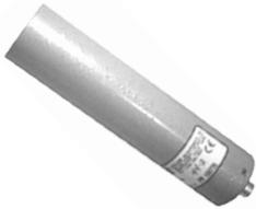
The response kit sodium iodide (NaI) gamma scintillator (Model 44-2) is used for the detection of low-level gamma radiation, in the range of 60 keV to 1.25 MeV. The detector is energy dependant, over-responding by a factor of 10 or greater in the 100 keV range, and under-responding by a factor of 0.5 above 1 MeV when normalized to  $^{137}\text{Cs}$ . The response of this detector is nominally linear (within 10% of true value), from 5  $\mu\text{R/hr}$  to 50 mR/hr.
