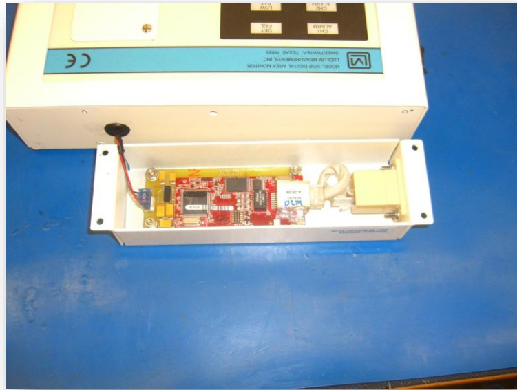
Figure 41 – External Rabbit Ethernet Board Removal
