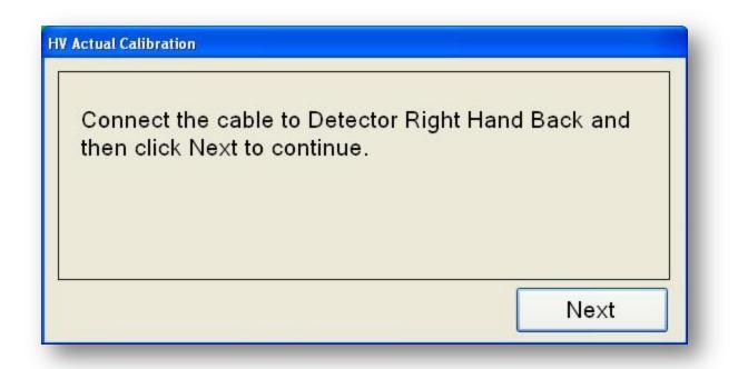
After connecting the cable and clicking the Next button, the high voltage will be restored to the set point. Enter the measured high voltage and click Next. Continue repeating this process until all detectors are completed.
