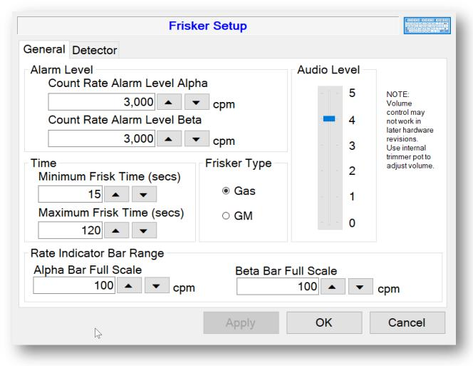
The General Frisker tab allows the setting of basic values that govern frisker operation. These values include the frisker Alarm Level, Audio Level, Time requirements, Frisker Type and Count Rate Indicator Bar Range.
