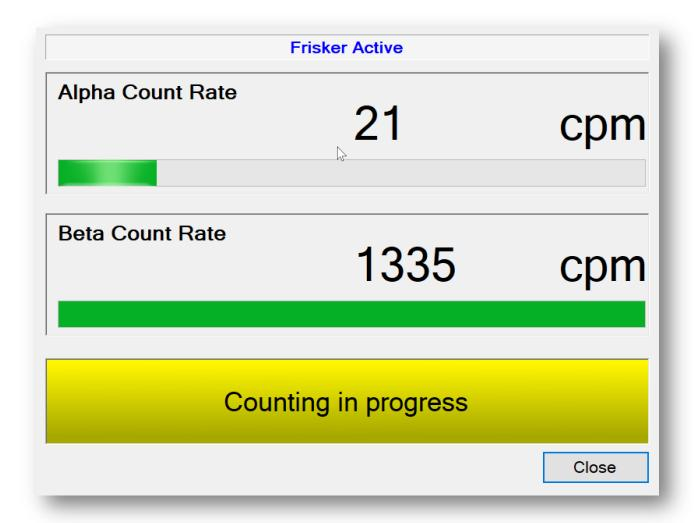
The Frisker Active screen displays a status bar at the bottom of the screen with digitial and bar type count rate indicators for all channels at the top of the screen. If at any time during the frisking operation the count rate exceeds the set limit, the background of that section turns red, along with illuminating the red stack light if equipped. The Close button in the lower right corner can be used to close the Frisker Active screen, but Level 1 or 2 password access is required.
