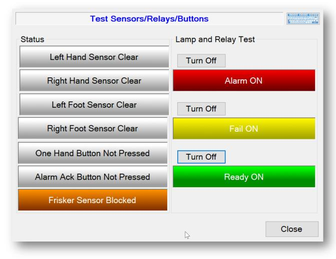
The outputs include the lights in the stack, relays, and infrared sensors. The inputs include the infrared sensors and pushbuttons. Click on the buttons to turn on/off the lights/relays. When a pushbutton is pressed, the indicator should light up to indicate the button was read successfully. The Model 4906
