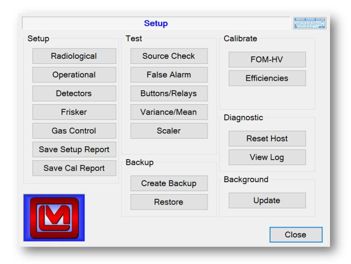
Radiological – sets up the counting mode and its parameters, background alarms, and units of measurement.
