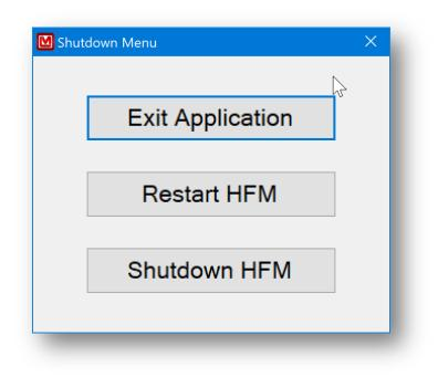
Exit Supervisor – closes the Supervisor application and provides access to the Windows 7 Pro environment. This is necessary for performing software updates, configuring windows settings such as printing or networking, or to provide access to the data files. A confirmation window will be displayed before the Supervisor application is closed.
