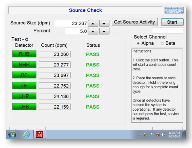
For two channel systems, select the appropriate channel for the source check (alpha or beta). Enter the source size of the check source and a percentage that the counts must fall within to be considered acceptable.
