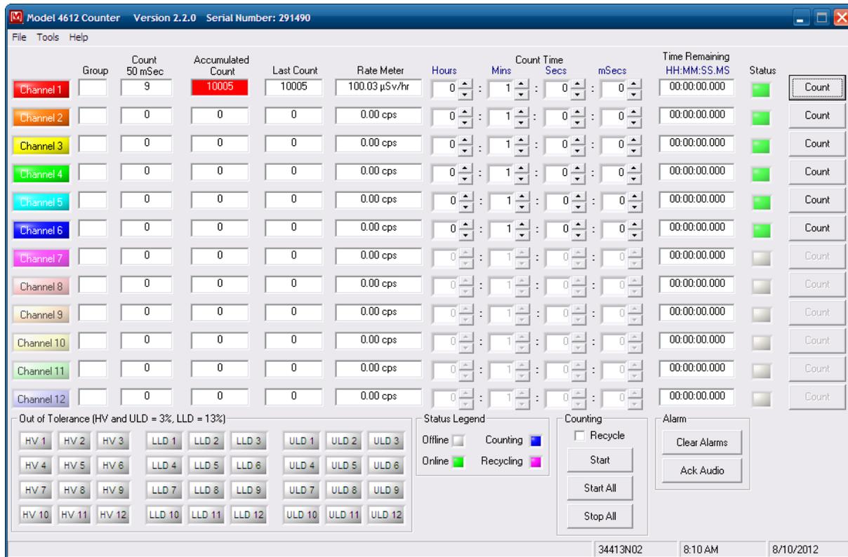
The main screen displays the following information: Group Number, current 50 millisecond count, Accumulated Count, Last Count, Count Time, Remaining Time, Status, and Out of Tolerance.
