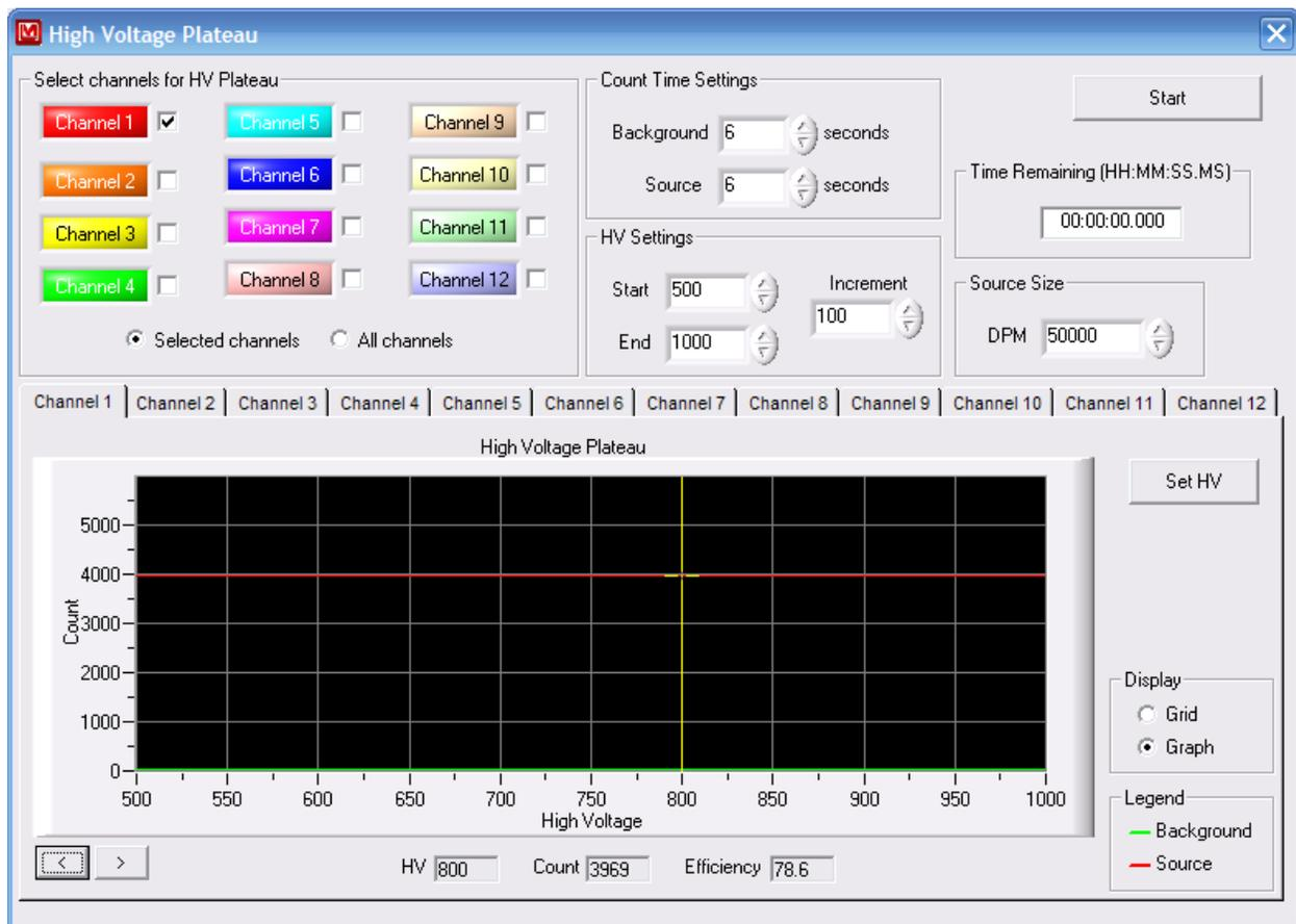
Once the plateau is complete, clicking on the Set HV button will set the high voltage and efficiency for the channel. Select the appropriate high voltage and efficiency by highlighting the row on the grid or by selecting a point on the graph with the cursor. On the graph view, the cursor can be moved by dragging it around the plot with the mouse or by using the Cursor Left and Cursor Right buttons, which are located at the bottom, left corner of the graph.
