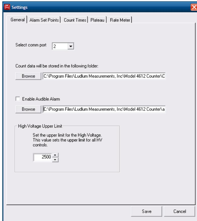
**Comm Port:** the RS-232 serial port used to communicate with the Counter. This list box displays all available communication ports on the computer. If a USB to serial adapter is used, consult the documentation that came with it for instructions on installing any drivers and configuring the port. The software will only work with communication port numbers that are between 1 and 16. If the port number is higher than this, it must be reconfigured to a lower number.
