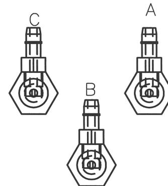
BARBS ARE LABELED FOR INSTALLING 1/4" TUBING
