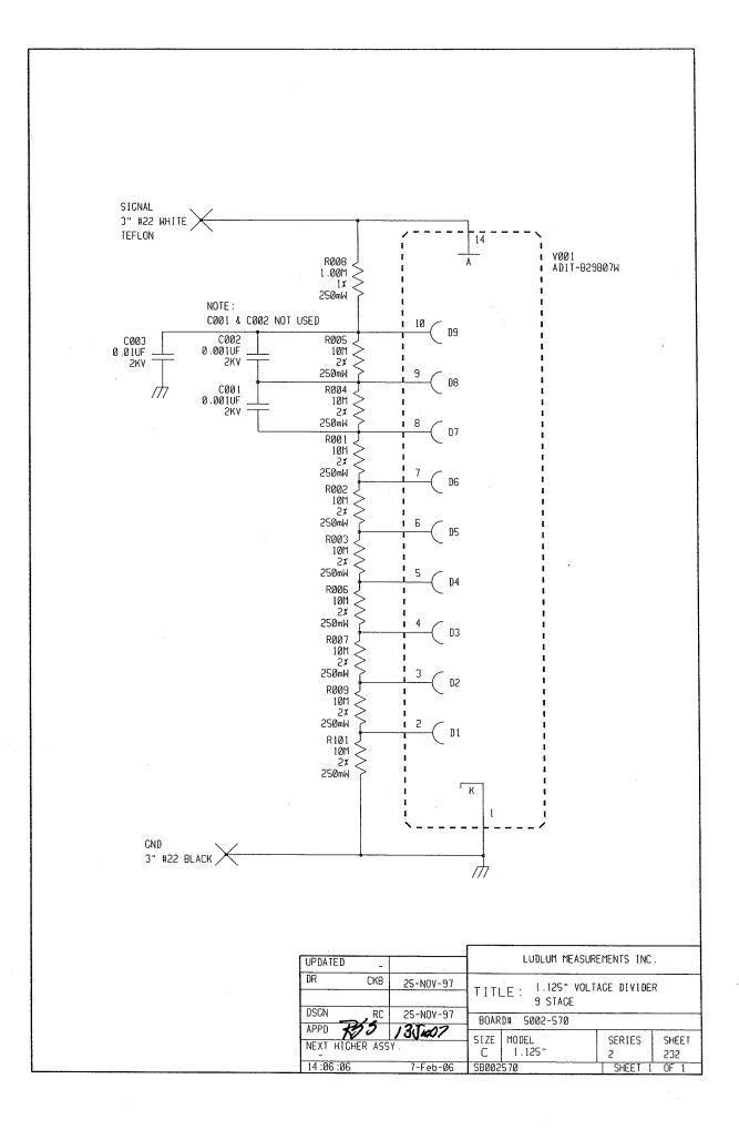
NOTE : COOI ,COO2 NOT USED 0 Ο ×CØØ2 R00 ×C00 RØØP C003 RØØ 1 0.010 RØØ2 101 , RØØ9 RØØ: D R007 Φ RØØ6 0 V001 ADIT-829807W LUDLUM MEASUREMENTS INC. SWEETWATER, TX. DR CKB Ø3-DEC-97 TITLE: 9 STACE VOLTAGE DIVIDER
