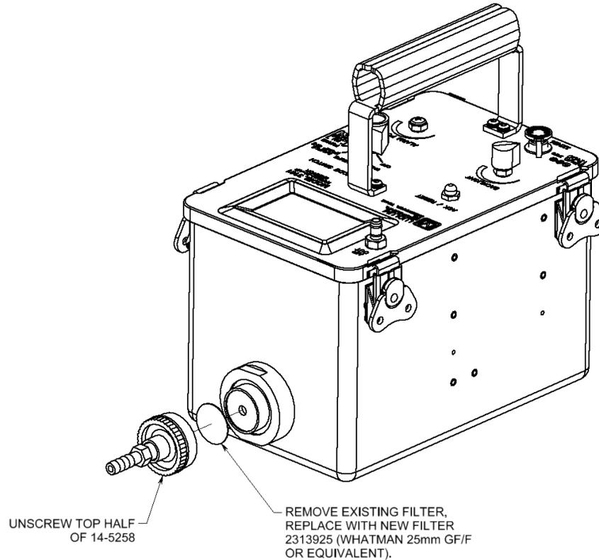
**Figure 4-2. Particulate Filter.**
