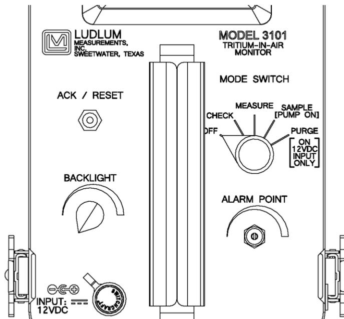
**Figure 2-1. Identification of Controls.**
