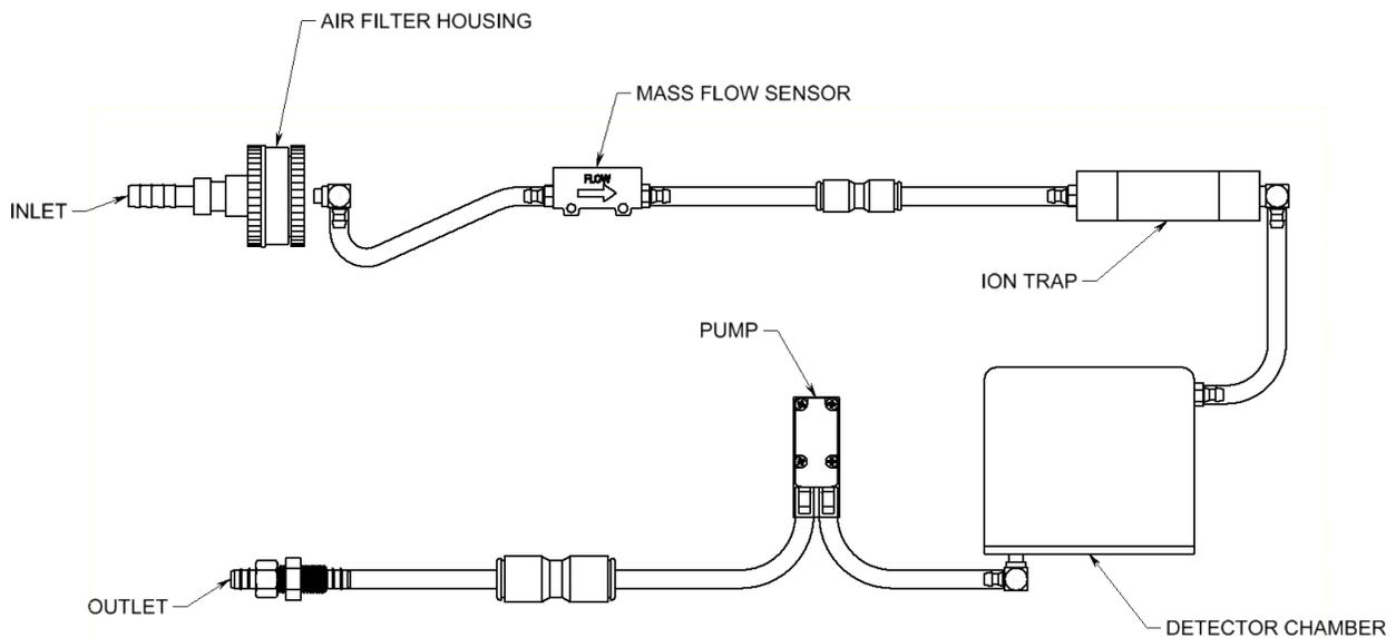
Figure 4-3. Air Flow Diagram.
