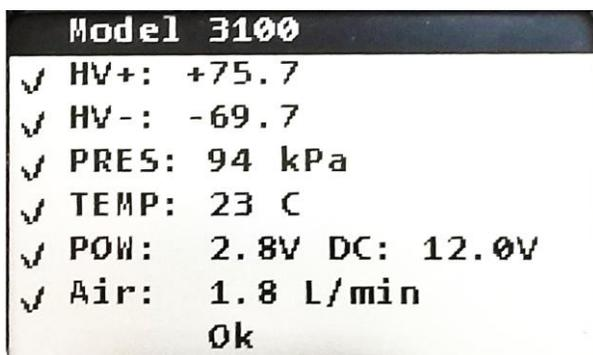
Figure 2-2. First Check Display Screen.
