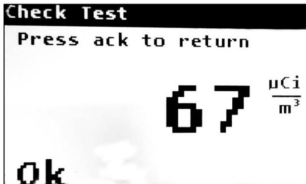
Figure 2-3. Check Test Screen Ok.
