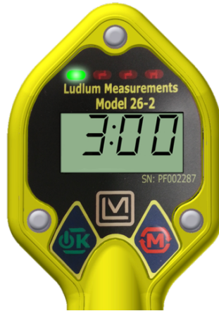
Figure 2.6: TIMED FRISK mode operation showing Frisk Timer of 3 minutes. Green LED will be steady ON.
