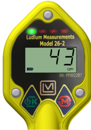
Figure 2.4: RATE mode display showing typical background radiation rate and the low-battery icon. Green LED will be flashing.
