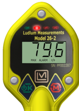
Figure 2.5: MAX mode operation display with ALARM indicators for Lowest Alarm Level. A single red LED will be flashing.
