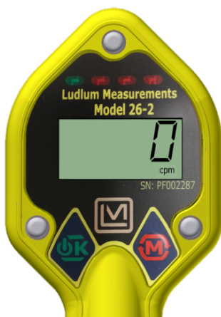
Figure 2.2: Detector Failure display (shown for cpm); will also flash.
