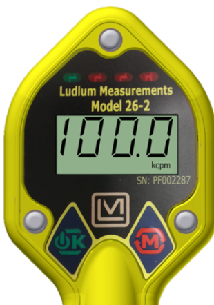
Figure 2.3: Detector Over Range (shown for cpm); will also flash.
