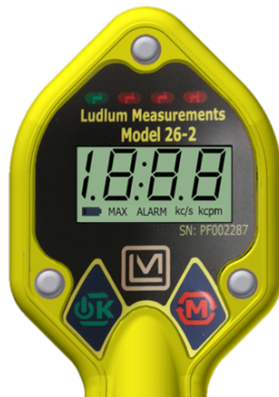
Figure 2.1: Startup display for the Model 26-2, with all LCD segments shown.
