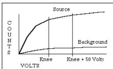
**Scintillators**: Set the DISC for 10 millivolts. Plot background and source counts versus HV to produce a plateau graph similar to the one in the figure. Adjust the HV to 25-50 volts above the knee or start of the plateau. This provides the most stable operating point for the detector.
