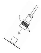
Connect a detector to the Model 2241-3 by using the cable provided; firmly pushing the connectors together while twisting clockwise until the connector latches (one-quarter turn). The diagram to the left illustrates how this is done. Next, place the detector selector switch in the appropriate position.
