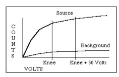
**Scintillators**: Set the DISC for 10 millivolts. Plot background and source counts versus HV to produce a plateau graph similar to the one in the figure. Adjust the HV to 25-50 volts above the knee or start of the plateau. This provides the most stable operating point for the detector.
