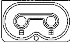
Install two "D" size batteries in the compartment. Note the (+) and (-) marks inside the battery door. Match the battery polarity to these marks. Close the battery box lid.
