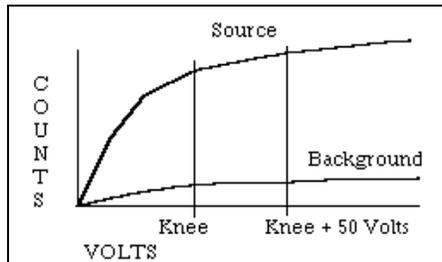
figure below. Refine the HV adjustment for optimum source efficiency with a minimum acceptable background count.
