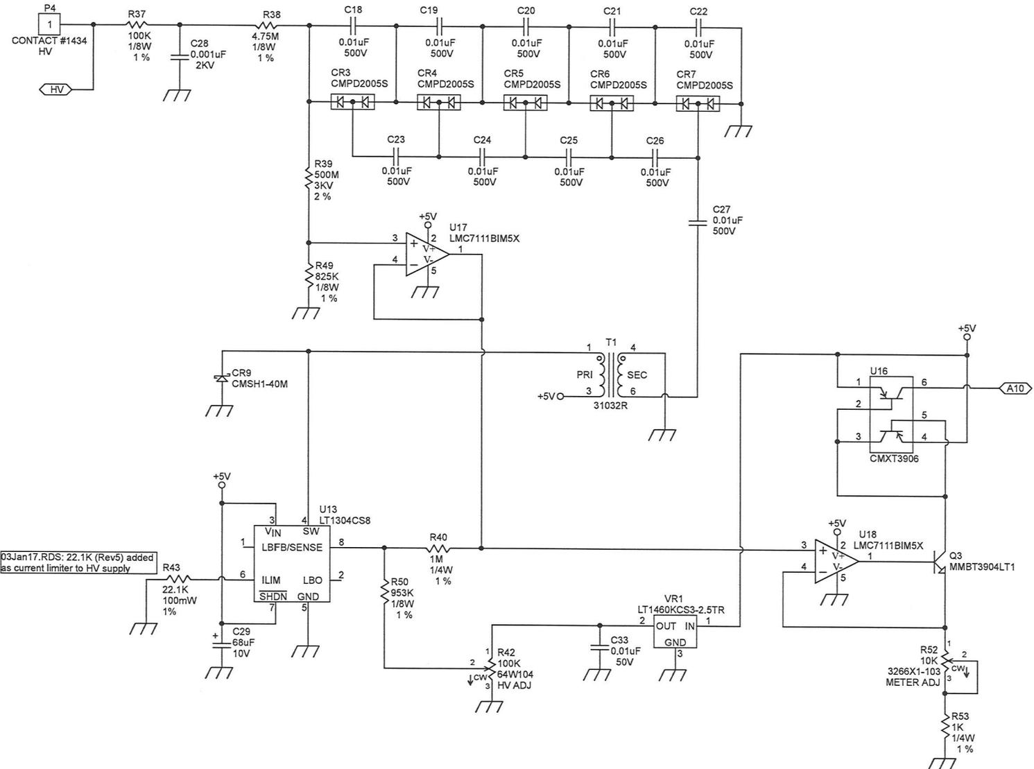
03Jan17.RDS: 22.1K (Rev5) added as current limiter to HV supply
