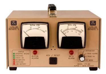
The radiation level is displayed on two analog meters. The Alpha meter dial indicates 0-1000 cpm on a three-decade log scale. The Beta meter dial indicates 0-100,000 cpm on a three-decade log scale. Each channel has its own distinguishable click-per-event audible tone. Beta events are a low pitch and alpha events are a high pitch. Beta clicks-per-event can be set at 1 per 1, 10, 100, or 1000.
