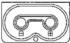
Note the (+) and (-) marks inside the battery door. Match the battery polarity to these marks. Close the battery box lid, push down, and turn the quarter-turn thumb screw clockwise a fourth of a turn.
