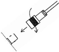
Connect one end of a detector cable to the detector by firmly pushing the connectors together while twisting clockwise a fourth of a turn. Repeat the process in the same manner with the other end of the cable and the instrument.
