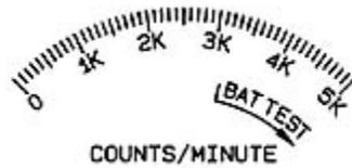
If the needle is pointing as indicated below and the instrument range selection switch is on the  $\times 0.1$  scale multiple, then the reading is 3.5 kcpm (multiplied by)  $\times 0.1 = 350$  cpm.
