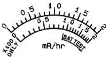
If the needle is pointing as indicated below and the range selection switch is on the  $\times 0.1$  scale, then the reading is 0.1 mR/hr.
