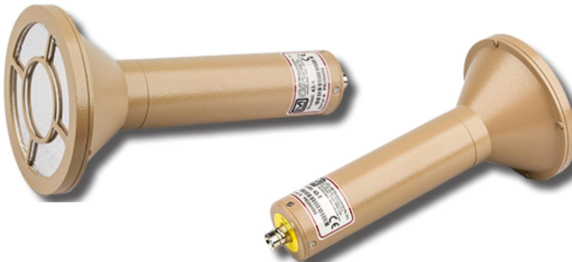
Two views to show the large window and the yellow to indicate the radiation type detected - in this case, yellow for alpha.
